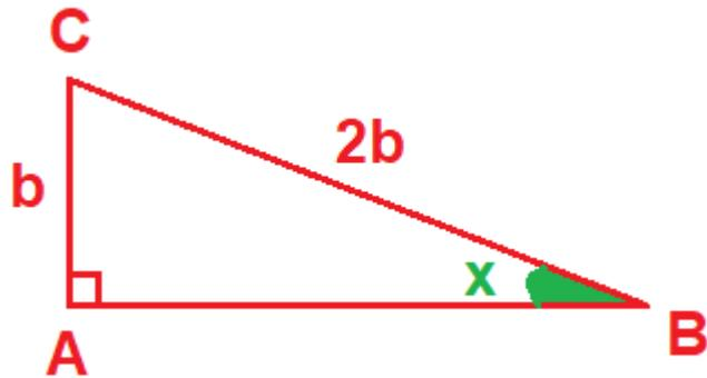
$$\text{sen } x = \frac{b}{2b} \rightarrow \text{sen } x = \frac{1}{2} \rightarrow 0^\circ < x < 90^\circ \rightarrow x = 30^\circ$$
